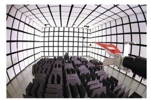
Figure 2-3. EMC Testing Chamber
